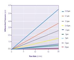
\*Flow rate is for a 25.4 cm (10 in) cartridge. For liquids other than water, multiply differential pressure by fluid viscosity (cP).
