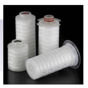
Biofil™ 2 Junior cartridges are based on a naturally hydrophilic polyethersulfone membrane with a mirrored asymmetric pore structure. When combined with quality all-polypropylene cartridge components and high integrity manufacturing techniques, the polyethersulfone membrane provides a high strength, long life cartridge of consistently precise microbial retention.
